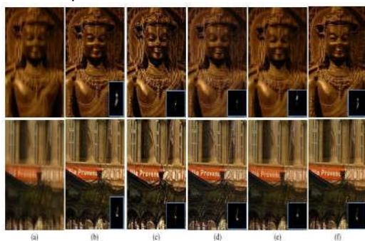
Fig5: Visual comparison of state-of-the-art methods. These two blurry images in (a) are from [21]. (a) Blurry images. (b) Xu and Jia [21]. (c) Krishnan et al. [4]. (d) Xu et al. [6]. (e) Zhong et al. [44]. (f) Our results
