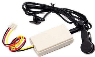
Fig6: Bluetooth module Heart beat sensor: The transmitter module includes three sensors. All three of these sensors can be found on the Heartbeat Sensor. When a finger is placed on it, this sensor produces a digital readout of the heart rate. The beat LED glows in time with each heartbeat while the heart beat detector is operational. It is possible to link this digital output directly to a microcontroller in order to measure the BPM rate. Light is modulated by the blood flow through the finger at each pulse, and this is how it works.
